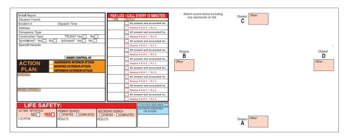
This Incident Command System consists of two tactical command worksheets mounted in a weatherproof case with built in legs. The worksheets have a dry erase surface that accepts magnetic tags that represent the Officers and apparatus at the incident. The Incident Commander will use the system to track the tactics and assignments throughout the duration of the incident.
