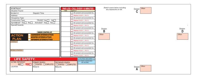
This Incident Command System consists of two tactical command worksheets mounted in a weatherproof case with built in legs. The worksheets have a dry erase surface that accepts magnetic tags that represent the Officers, tasks and apparatus at the incident. The Incident Commander will use the system to track the tactics and assignments throughout the duration of the incident. Custom layouts are available.
